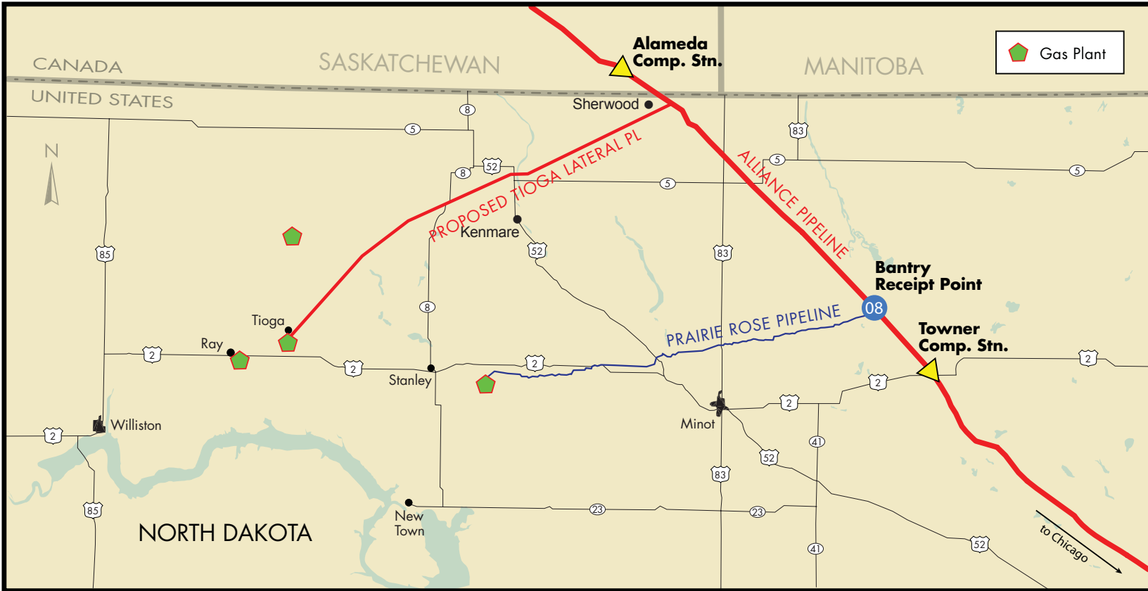
The 77-mile pipeline will transport Bakken natural gas from Tioga to enter a mainline near Sherwood.
